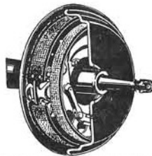
Fig. 51. Rear wheel brake showing the two-in-one brake drums.
