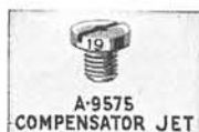
Fig. 13. Compensating jet: This jet (F, Fig. 10), empties into the compensating well which is opened to the air, and therefore is not subject to suction. Its flow of fuel is constant, being determined by the fuel level in the bowl and the size of the jet. It is most effective at low speeds. Size No. 19.
