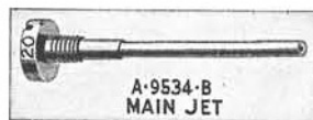
Fig. 12. Main jet: This jet (E, Fig. 10), is directly connected with the fuel chamber, being subject to suction its flow of fuel will vary with the load or speed of the engine. Its effect is most noticeable at high speeds. Size No. 20.
