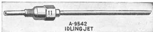
Fig. 15. Idling jet: Its function (D, Fig. 10), is to measure the fuel for closed throttle (idling) operation. When the throttle is opened, it is put out of action as the fuel then changes direction and goes through the cap jet. Size No. 11.
